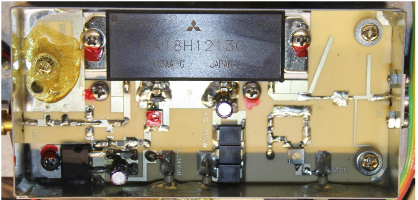
This transmitter has the DG0VE RA18H1213G 20 watt PA
